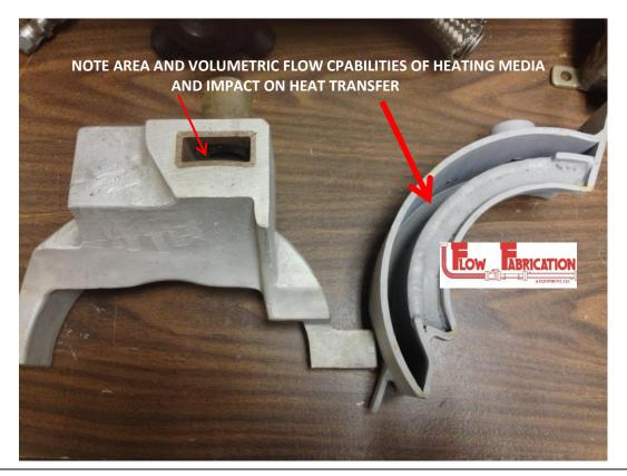
Clamp on / Bolt on jackets cross-sections. **Flow Fab** on Right side of picture, competitor with aluminum body and steel insert on left side of picture.
