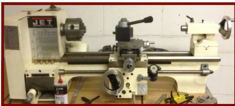
Lathe for machining valve seats
