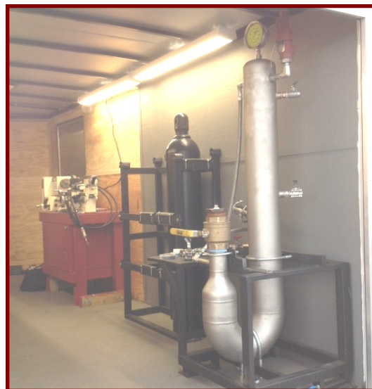
J-Tube testing device shown on right
